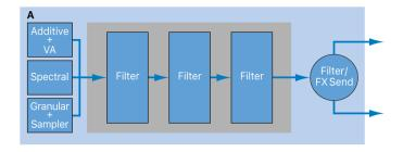
• When the source filters are configured in parallel, the signal is split and fed through the three filters simultaneously.
