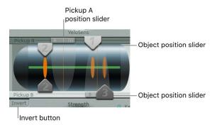
The green horizontal line within the Pickup display represents the string. As the Stiffness parameter value of the string is increased, the line becomes thicker. The line can be animated and can show the range of string motion.
