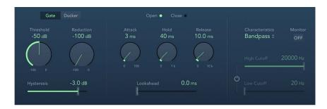
Unwanted triggering by low or high frequency noise is avoided by the dedicated sidechain filters of the Noise Gate plug-in.
