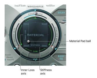
The four corners of the Material Pad display different material names. These each represent a combination of maximum/minimum Stiffness and Inner Loss values. The combination of the Inner Loss and Stiffness parameter positions determine the string material and, therefore, the general timbre of your sound. Here are examples of how Inner Loss and Stiffness settings can change the tonal color:
