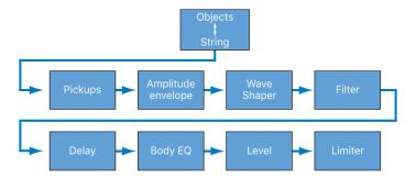
This figure shows the signal flow of the core Sculpture synthesis engine.
