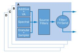
Each source provides multiple sound generating elements based on different methods of synthesis. See Source elements overview.
