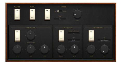
The default effect signal flow is as follows: the organ signal runs through the Equalizer, Wah, and Distortion effects. This treated signal is then fed into the Reverb and finally passed to the Leslie rotor effect.
