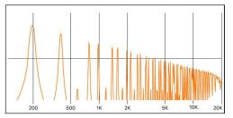
The square wave can be reshaped to make the waveform cycles, or pulses, more rectangular, by using a *pulse width modulation* (PWM) control. The more rectangular the wave becomes, the more nasal it sounds. When modulated in this way, the square wave is known as a *pulse wave*, and contains fewer harmonics. It can be used for reeds, basses, and brass sounds.
