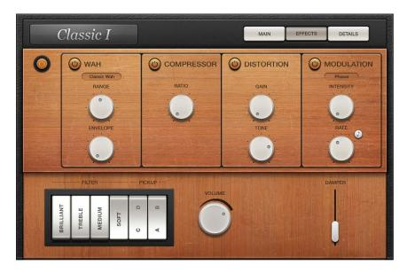
Vintage Clav effects work in series—where the output of one effect is fed into the next in an effects chain. The routing order lets you choose whether a distorted signal should be wah-filtered (for funkier sounds) or the wah-filtered sound should be distorted (for screaming sounds)—as an example.
