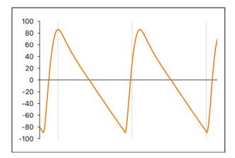
This example illustrates how using a filter to cut away portions of the frequency spectrum alters the waveform shape, thus changing the timbre of the sound.
