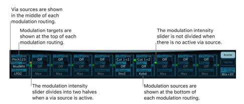
Any modulation source can be connected to any modulation target, much like an old-fashioned telephone exchange or a studio patch bay.
