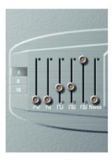
In addition to triangular, sawtooth, and rectangular waves, the rectangular waves of two sub-oscillators are also available. The left sub-oscillator fader is one octave lower than the main oscillators, and the right sub-oscillator fader is two octaves lower. Use these to fatten up the sound.
