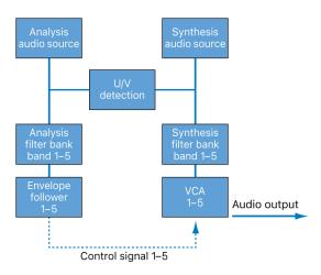
The more bands a vocoder offers, the more precisely the original sound character is reproduced by the synthesis filter bank. EVOC 20 PS provides up to 20 bands per bank. See EVOC 20 block diagram for a detailed image of the EVOC 20 PS signal path.
