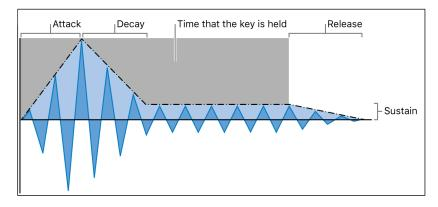
The envelope generator usually features four controls—Attack, Decay, Sustain, and Release, commonly abbreviated as *ADSR*.
