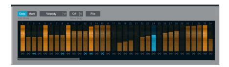
Step edit mode: In Step edit mode, you can view and edit the sequence one parameter at a time, with step values displayed as vertical bars. Drag vertically to edit step levels. Option-click to reset a step to zero.
