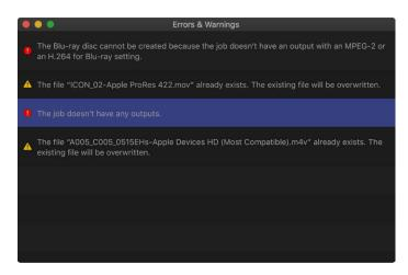
In the Errors & Warnings window, click an alert message to highlight the affected job in the batch area. Alerts showing a yellow yield sign  $\triangle$  are warnings that won't prevent a batch from being started but may result in errors or unexpected results. Alerts showing a red stop sign  $\bigcirc$  are errors that must be fixed before a batch can be started.
