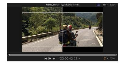
*Padding* doesn't remove any of the source image. Instead, padding adds black to the image to fit it into a different-size frame. This can be useful for transcoding files that are stored with incorrect pixel aspect ratios, such as widescreen DV files that appear squished. You can also use the padding controls to shrink an image and deliberately add black borders around the outside of the image.
