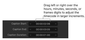
• Change the start point or end point to a precise value: Select the hours, minutes, seconds, or frames area of timecode in the Caption Start or Caption End field, enter a new two-digit number, then press return.
