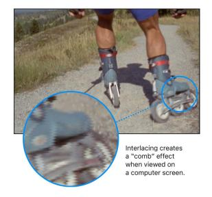
You can *deinterlace*, or remove the fields from an interlaced video clip, by converting it to a progressive frame rate. The video settings provided in Compressor contain a "Field order" pop-up menu in the Video inspector that you can use to turn interlacing on or off for the transcoded file. For more information, see the topic that covers the format you're using for transcoding, for example, QuickTime Movie or MPEG-2.
