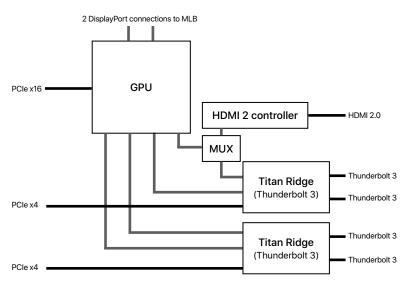
Radeon Pro W5700X MPX Module architecture
