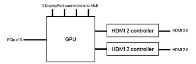
Radeon Pro 580X MPX Module architecture
