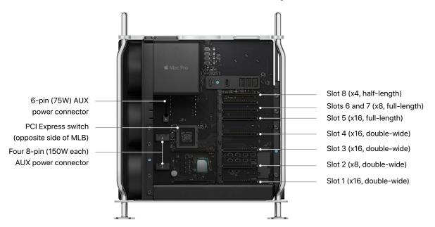
Mac Pro provides four 8-pin auxiliary (AUX) power connectors that each provide 150W of power, for a total of 600W of AUX power. This power is in addition to the 75W of power provided directly by each PCle slot. Combined, up to four 225W graphics cards can be installed in Mac Pro, each in an x16 slot with a total power of 900W. A single 6-pin AUX power connector provides 75W of additional power for PCle cards in slots 5, 6, and 7.
