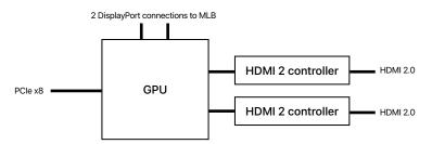
Radeon Pro W5500X MPX Module architecture
