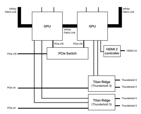
Radeon Pro W6800X Duo MPX Module architecture
