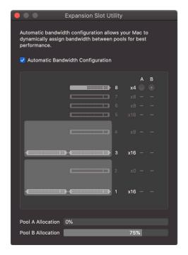
**Expansion Slot Utility** showing two MPX Modules installed, represented by the gray boxes, and the default Automatic Bandwidth Configuration selected.
